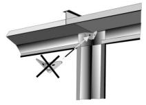
For the connection of the unit elements at the base frame, use the supplied M8 x 30 or M10 x 30 hex head screws. No brackets are used at these points.
