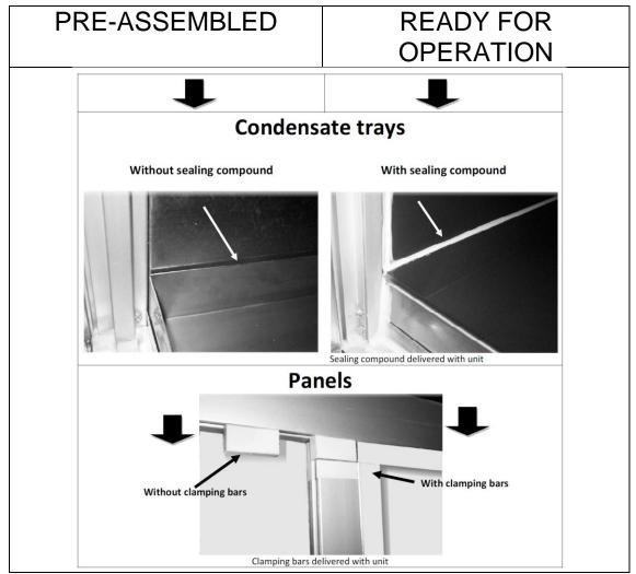
All panels must be secured on all sides with the supplied clamping bars.
